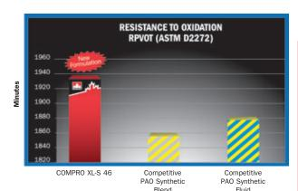
New and Improved COMPRO XL-S provides stronger resistance to oxidative breakdown than the competitive products tested.
