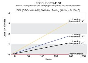
In the DKA oxidation test, product performance is measured by how much the acidity of the oil (TAN) increases over time (therefore the flatter the line the better.) Compared to the leading competitors, Petro-Canada's PRODURO TO-4' 30 ad vanced formulation resists oil degradation best.
