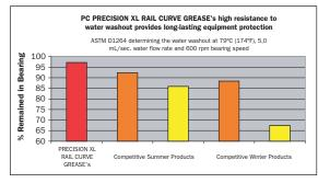
\*This standard grease industry test demonstrates the water resistance of PRECISION XL RAIL CURVE GREASE in wet conditions.
