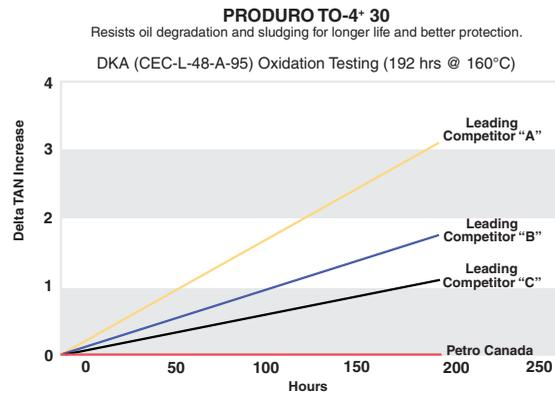
In the DKA oxidation test, product performance is measured by how much the acidity of the oil (TAN) increases over time (therefore the flatter the line the better.) Compared to the leading competitors, Petro-Canada's PRODURO TO-4<sup>+</sup> 30 advanced formulation resists oil degradation best.
